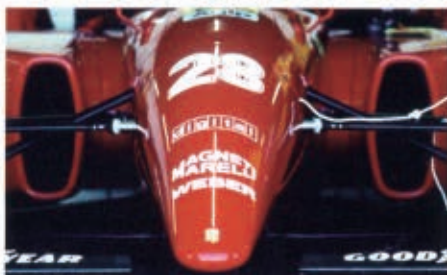
TWIN TUNNELS: Pods housing radiators connect to central chassis through small wing sections.
